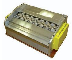
Industrial Magnetizers: Flexmag manufactures several industrial units in widths from 13" up to 26". These motorized magnetizers have a variable speed control that runs up to 145 feet per minute, and they will permanently magnetize substrates up to .060" thick - both standard and high energy.
